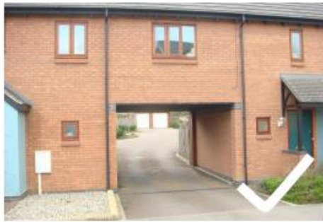
"Bridge over unit" makes a clearer definition that the rear court is private
